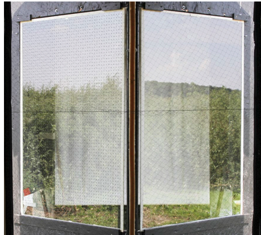
Despite the small spacing between dots, this dot grid is ineffective: a dense grid of black dots with 3mm diameter was not recognised by birds even on surface 1 (left: test pane, right: reference pane).
