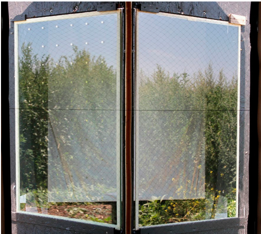
Eastman Saflex® FlySafe™ SEEN shiny 9/90: metallic dots, 9mm in diameter and 90mm apart: highly effective and – due to high reflectance – also suitable for surface 2 (left: test pane, right: reference pane).
