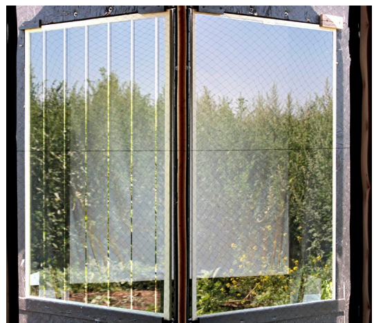
Arnold Glas Ornilux® design lines 5/95: highly effective metal marking with classic striped pattern (left: test pane, right: reference pane).
