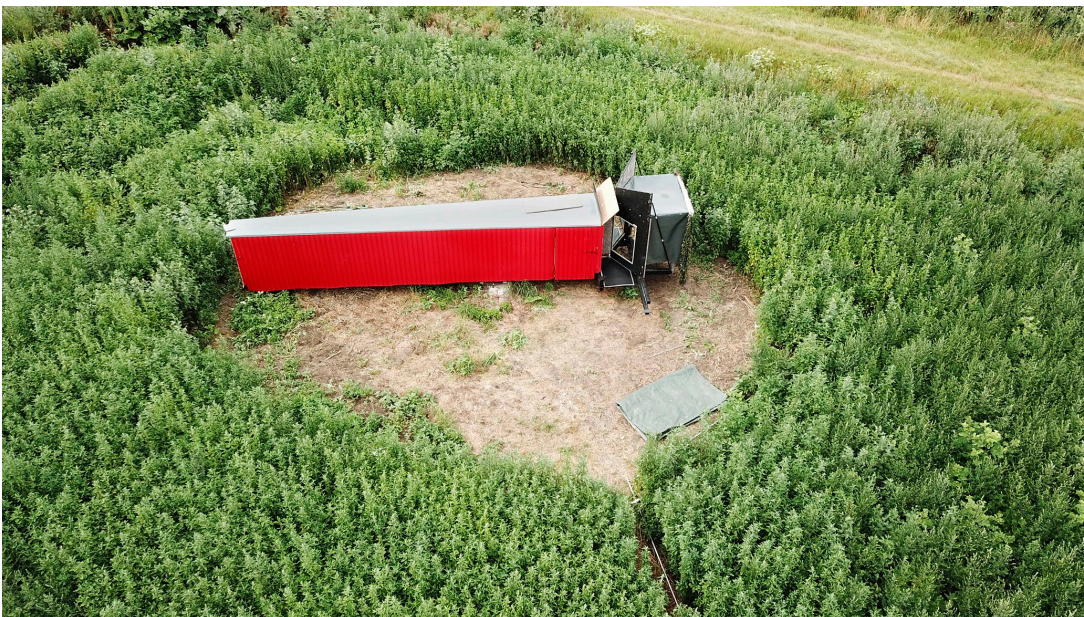
The flight tunnel of the Hohenau-Ringelsdorf Biological Station before the start of the research season, when the vegetation has not yet developed fully. The circular clearing corresponds to the rotation range of the test apparatus, which is mounted on a pivot so that the sun is always behind the birds. The birds are placed in the tunnel at the narrow end and immediately take off in the direction of the test panes (right). They are intercepted by a net, then released unharmed through the side door.
