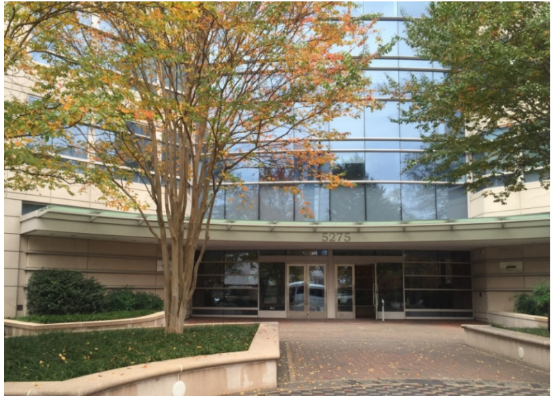
An example of where trees and shrubs are reflected in the glass and create a type of funnel effect near the entrance of a building. Photo by USFWS
